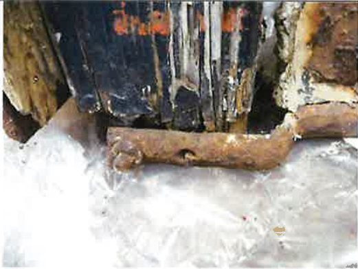
Detail of bottom edge of side B of pub sign showing corrosion through painted surfaces, before conservation
